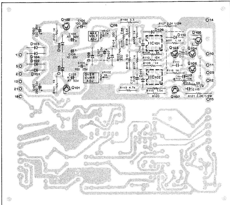
Q101 : 2SD400, Q102 : 2SB544, Q103 104,106,107 : 2SC983, Q105 : 2SD525, D101~104 : GP10-4002
